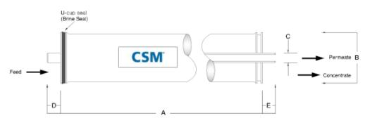
1. Each membrane element supplied with one brine seal, one interconnector (coupler) and four o-rings. 2. All R4021 elements fit nominal 4.0 inch (102 mm) I.D. pressure vessels.
